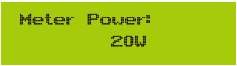
Pic 7.19 Zero-export function via energy meter turn on
