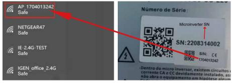
Microinverter SN: 2208314002 Built-in datalogger: 1704013242
