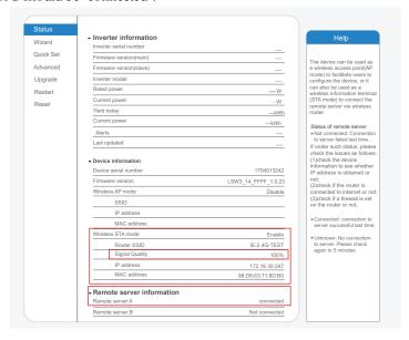
10. If both remote server A and B are "Not connected", please refresh the page or repeat the previous steps. If the "Signal Quality" is lower than 40%, please move your Router closer to the Microinverter.
