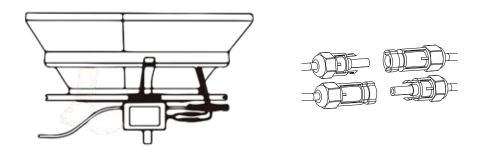
**NOTE**: When plugging in the DC cables, if AC already available, the Microinverter should immediately blink red light and will start work within the setting time (default 60 seconds). If AC is not available, the red light will blink 3 times quickly and repeat after one second until AC is connected.
