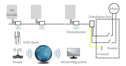
**NOTE**: If the wireless signal in the area where the microinverter is weak is weak, it is necessary to add a wifi signal booster at a suitable place between the router and the microinverter.
