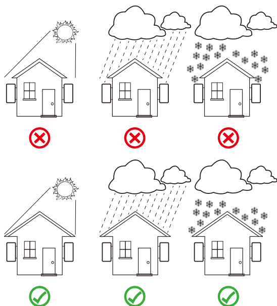
Pic 4.1 Recommended installation place
