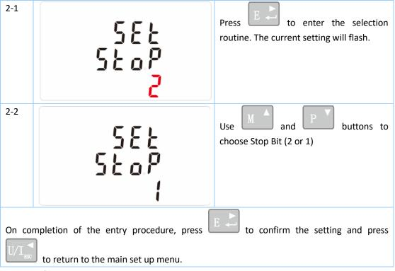
Note: Default is 1, and only when the parity is NONE that the stop bit can be changed to 2.
