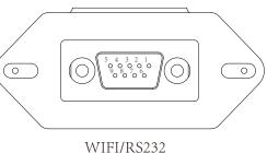
This RS232 port is used to connect the wifi datalogger
