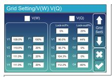
V(W): It is used to adjust the inverter active power according to the set grid voltage. V(Q): It is used to adjust the inverter reactive power according to the set grid voltage.
