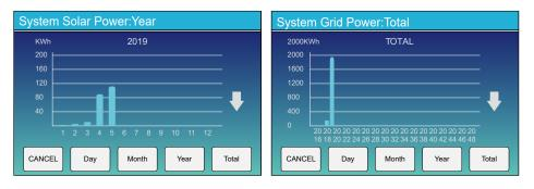
Solar power curve for daily, monthly, yearly and total can be roughly checked on the LCD, for more accuracy power generation, pls check on the monitoring system. Click the up and down arrow to check power curve of different period.
