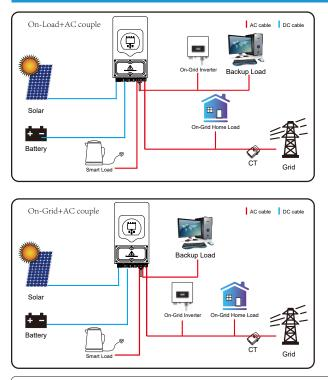
The 1st priority power of the system is always the PV power, then 2nd and 3rd priority power will be the battery bank or grid according to the settings. The last power backup will be the Generator if it is available.
