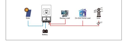
**Solar Sell:** "Solar sell" is for Zero export to load or Zero export to CT: when this item is active, the surplus energy can be sold back to grid. When it is active, PV Power source priority usage is as follows: load consumption and charge battery and feed into grid.
