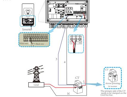
\*Note: when the reading of the load power on the LCD is not correct, please reverse the CT arrow.
