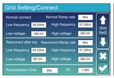
**Normal connect**: The allowed grid voltage/frequency range when the inverter first time connect to the grid. **Normal Ramp rate**: It is the startup power ramp.
