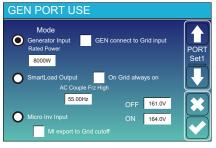
**Generator input rated power:** allowed Max. power from diesel
