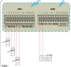
CT-R (1,2,7,8): current transformer (CT-R) for zero export to CT mode clamps on L1 when in three phase system.
