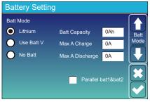
**Battery capacity:** it shows your battery bank size to Deve hybrid inverter.
