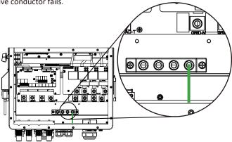
Earth Connection (Copper wires) (bypass)
