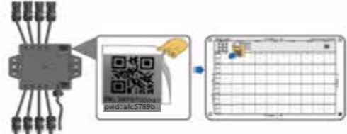
f. Schematic diagram of optimizer concentrator QR code tearing and pasting
