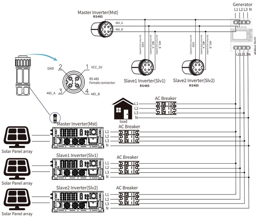
Pic 7.21 Eastron Connection diagram(The pass-through table)
