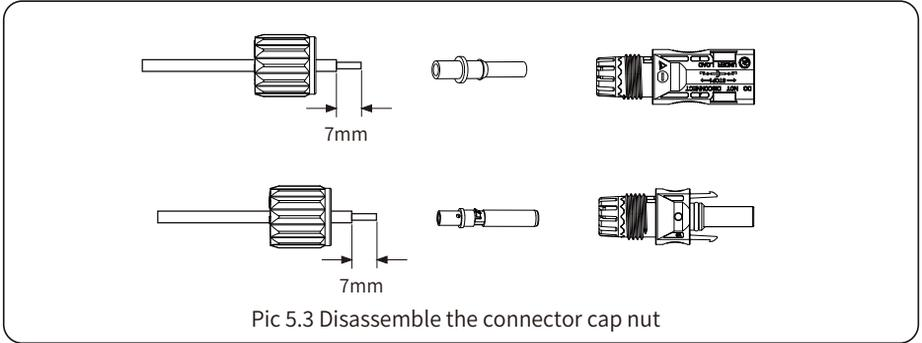
Pic 5.3 Disassemble the connector cap nut
