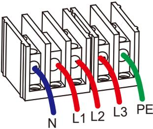
Pic 5.9 Connect AC wires to the terminals
