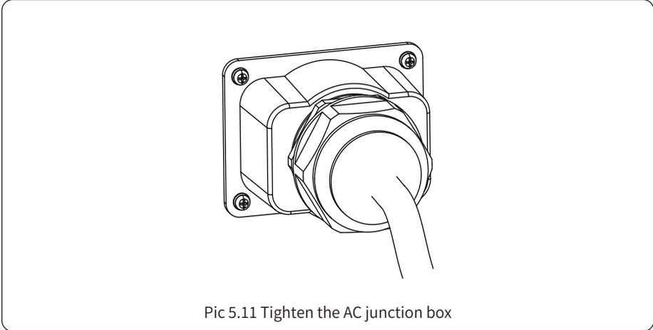
Pic 5.11 Tighten the AC junction box
