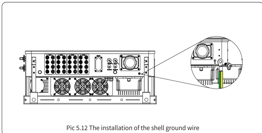
Pic 5.12 The installation of the shell ground wire
