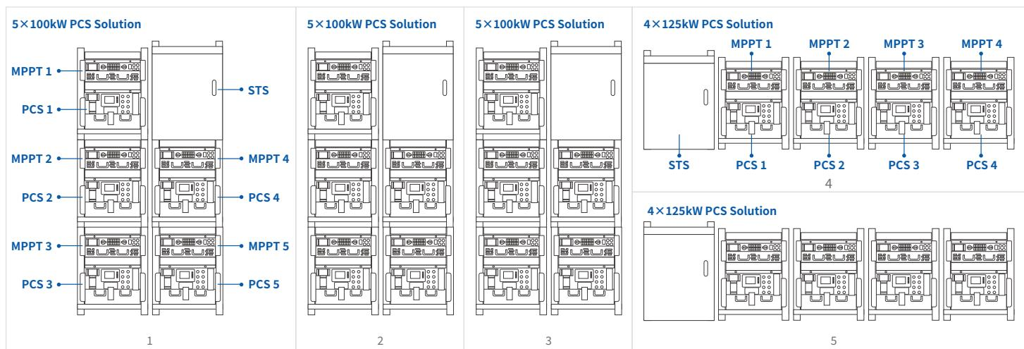
**Up to five STS modules can be paralleled to form a 2.5MW system**
