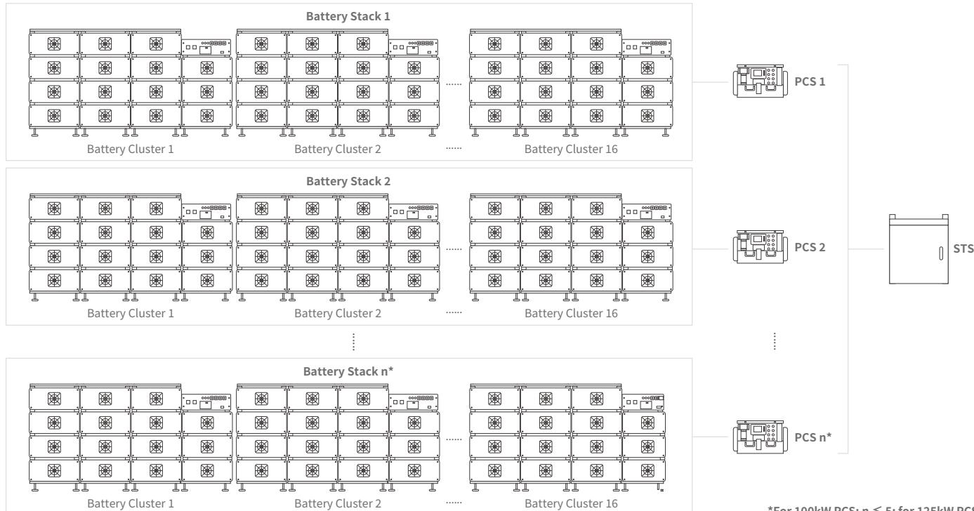
**One STS module can connect to five 100kW PCS modules or four 125kW PCS modules for parallel operation**
