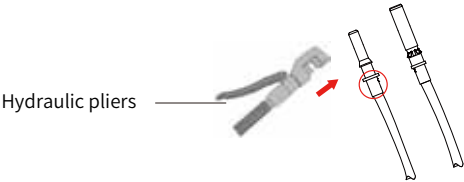
Pic 3.4 Crimp the contact pin to the wire
