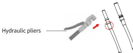
Pic 5.4 Crimp the contact pin to the wire
