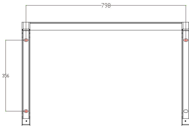
Pic 4.4 Mounting bracket dimensions
