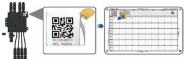
f. Schematic diagram of Concentrator Controller QR code tearing and pasting
